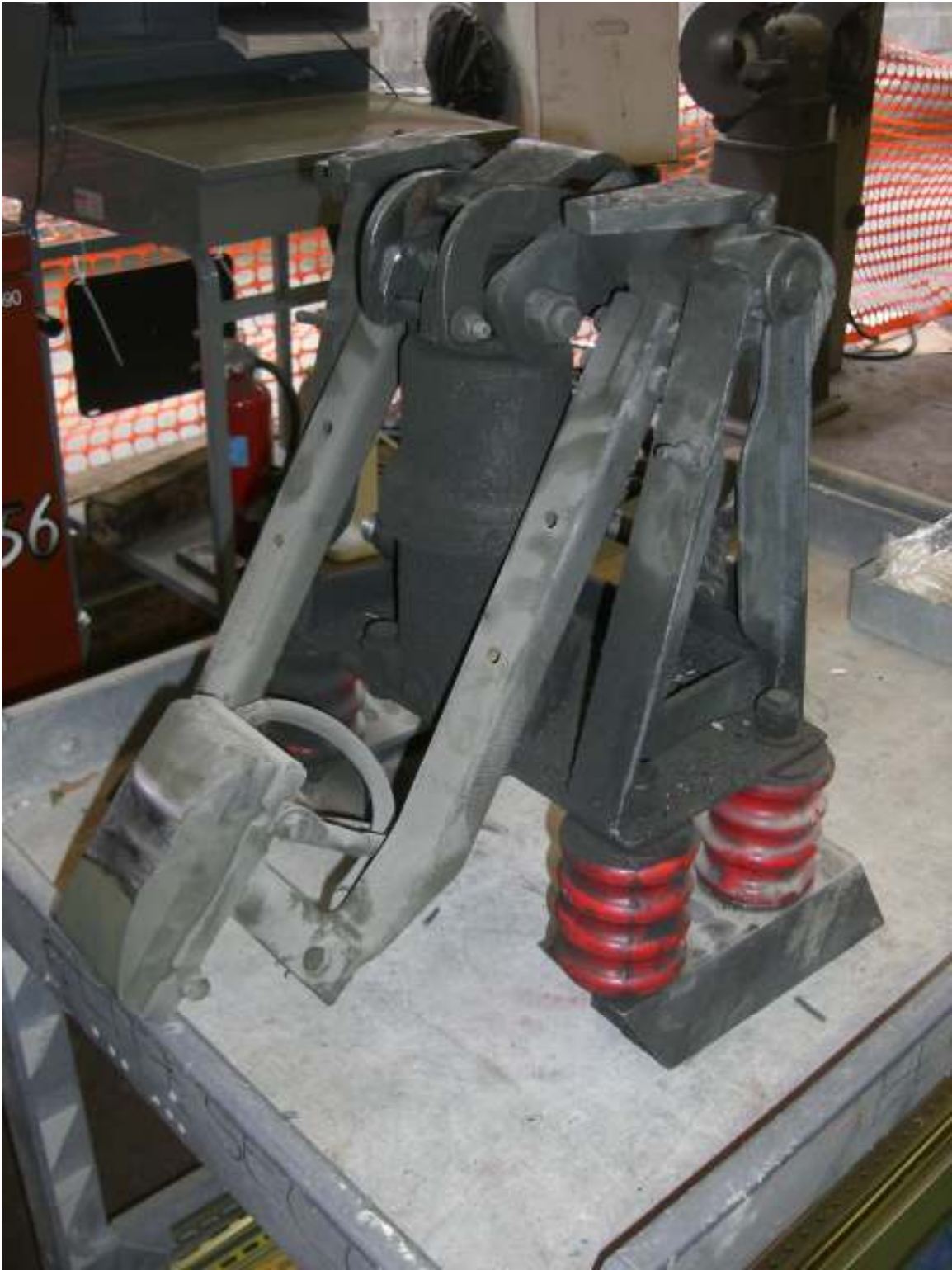
Positive Collector Assembly removed from train to show detail
