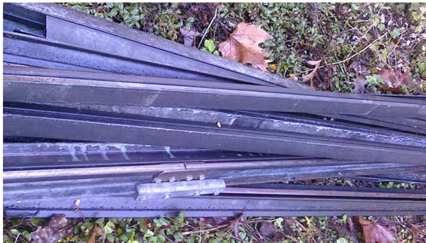
Copper-headed steel rail with joints cut and removed in 13.5-ft sections.
